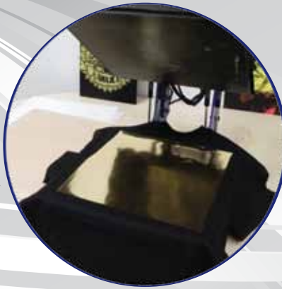
Step 2: Place foil over the print and cure with heat press.
